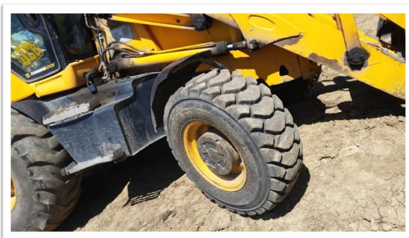
Hulk on the front axle and Super Industrial Lug in the rear axle of this JCB 3CX
