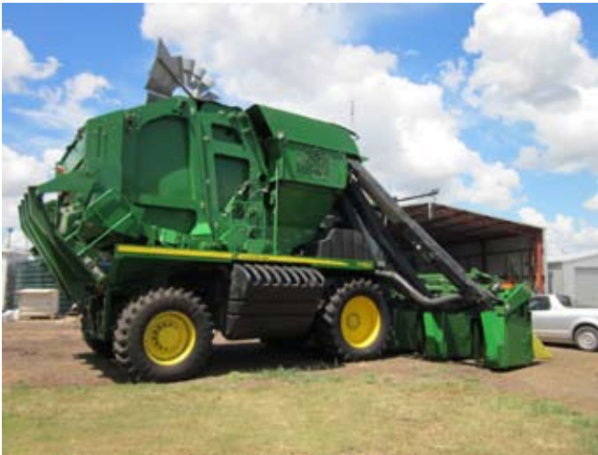
Jamie's John Deere with its recently mounted Alliance A360 - SUPER POWER DRIVE R-1 tires. The A360 are wide base radial tractor tires, developed for modern and high power machines on heavy duty field jobs.
