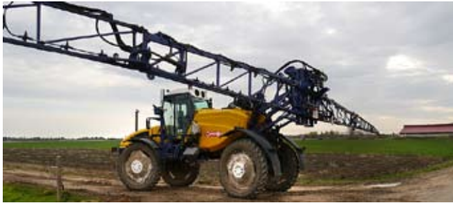
Alliance A350 were chosen by the OE; Optimized soil and row crop protection together with exceptional self cleaning characteristics.
