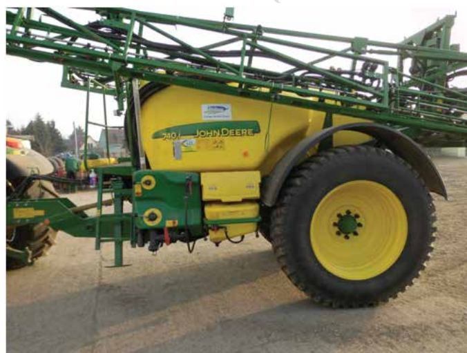
Alliance 550 MULTIUSE , size 480/80R38. Machine - John Deere 740i, towed sprayer
