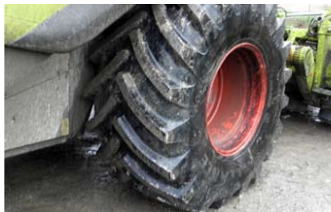
The A-375 mounted on a Claas Lexion 570C combine
