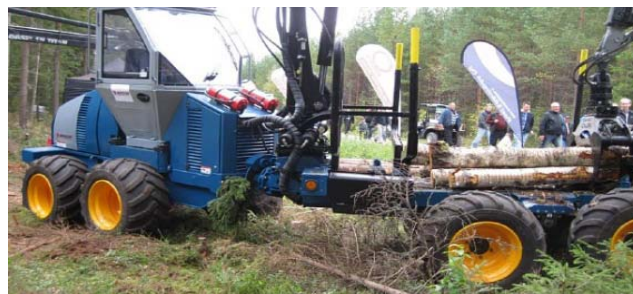
Novotný small Forwarder equipped with a full set of ALLIANCE 500/50-20 331 Heavy Duty
