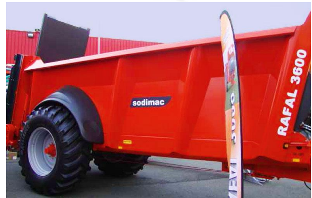
Alliance 710/70R38 178A8 A 360 tires on a Sodimac spreader, SPACE 2010
